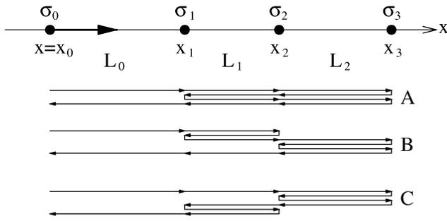
FIG. 1. Top: Quantum chain graph with vertices (dots) and bonds (line segments). The bold arrow shows the initial state used to compute the RP. Bottom: The family  $[m_0, m_1, m_2] = [1, 2, 2]$  of different but isometric orbits returning after topological time  $n = 10$  to the vertex 0.
